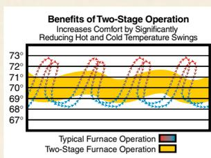
The QuietComfort® IIX 96 automatically adapts its operation to match your heating requirements. When the weather outside gets colder, the higher stage kicks in, increasing the speed of the circulation motor and the output of the burners to provide maximum warmth and comfort.
