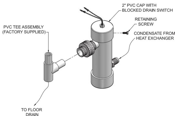
8. A condensate removal pump is required if the boiler is below the drain. When installing a condensate pump, select one approved for use with condensing boilers and furnaces. The pump should have an overflow switch to prevent property damage from condensate spillage. Call your qualified service technician to inspect the boiler and system.
